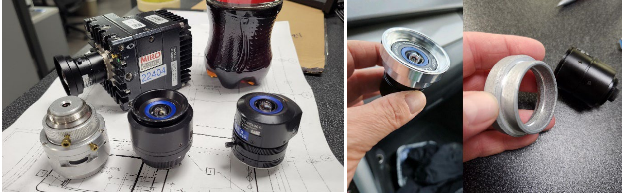
Figure 2. The left image shows Theia's ML183M, and the additional metal barrel, housing, and lens hood required for additional protection during crash testing. The right images show Theia's MY23F and the single additional component needed to protect the lens – the aluminum lens hood.
